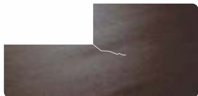
Cutting a laminate sheet at an angle of 90 degree leads to development of cracks in corner after pasting. Therefore it is advisable to avoid cutting at an angle of 90 degrees.
